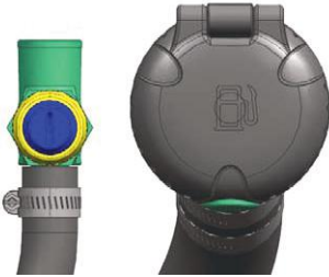
Figure 4-2. P-Trap and Deck Fill
