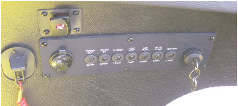
Figure 2-13. Circuit Breaker Panels
