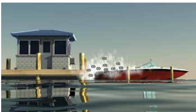
Blockage of boat exhaust by obstruction.
