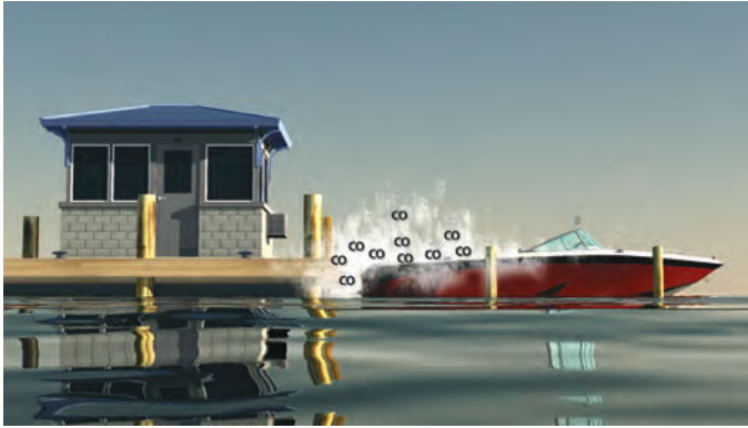
Blockage of boat exhaust by obstruction.
