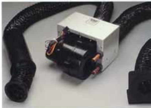
Two or Three outlet heaters with three speed control are available on all Malibu inboards.
