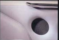
Stereo speakers are recessed in the side panels replacing plastic speaker grills for optimum form and function.
