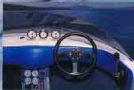
*Speedo and tachometer are placed perfectly on the dash for easier visibility. All other gauges and controls are placed within easy reach of the driver on a center console panel to the left of the foot well.*
