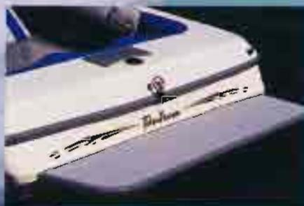
*The Tantrum's fiberglass swim platform accommodates full size sleds and is easily removed from the boat for tighter storage areas.*
