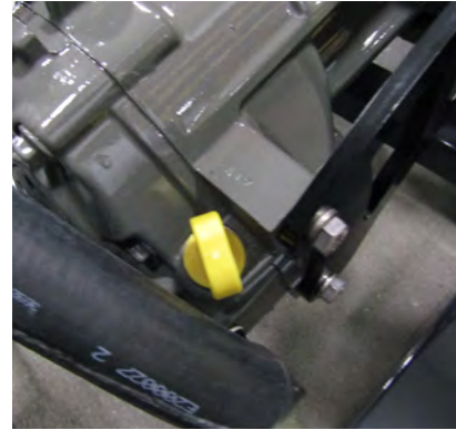
Transmission dipstick (red); V-Drive dipstick (yellow).
